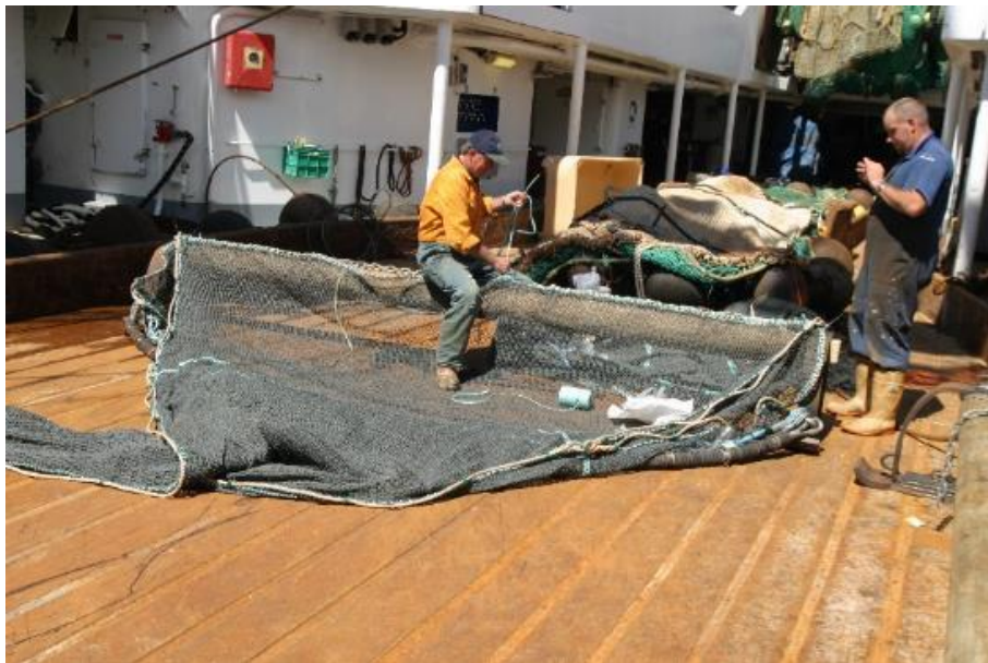
Figure 4-15: NIWA's beam trawl, a simple but effective sampling tool for benthic invertebrates.
