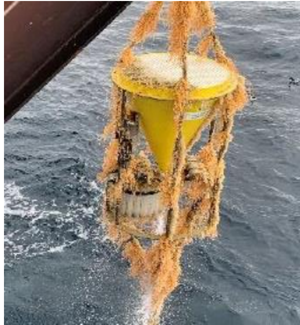
Figure 4-4: The 2019 mooring sediment trap, showing the extensive growth of hydroids after 12 months.
