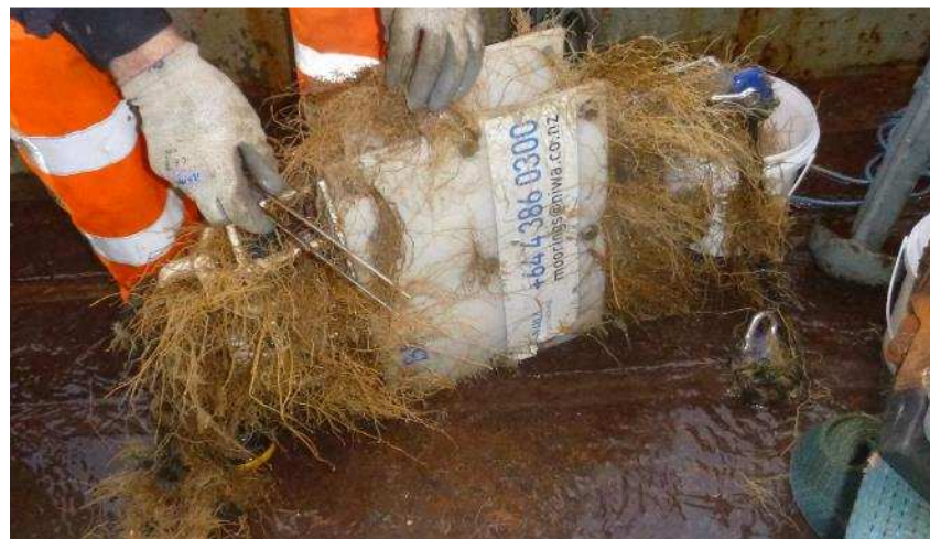
Figure 4-4: An acoustic release from the ADCP mooring, showing the extensive growth of hydroids after 12 months in the water.
